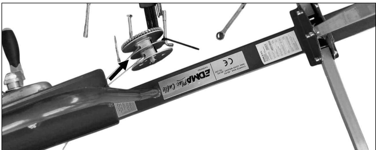
9. Push the cable to be replaced through the large opening on the hub. Unscrew the cable clamp and remove the worn cable from the winch.
