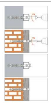
Screw-in the special screw until the head of the screw touches the sleeve; the anchor is correct mounted, if there is no turn-through of the plastic sleeve in the drill hole and if slightly move on turning of the screw is impossible
