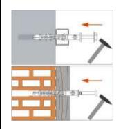
Insert the plastic sleeve and special screw into the hole through the fixture by slight hammer blows
